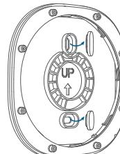
2. Install Siren's bracket on the wall with the screws provided.
