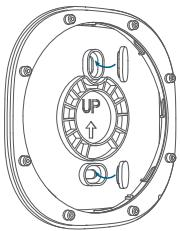
4. Position Siren on its bracket and twist clockwise to align the marks on the edge.
