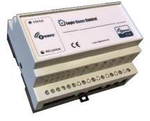
LHC5028 is a 6 channel Z-Wave controlled DIN mountable module. The module is equipped with 6 relay switches and 6 digital inputs for mounting on a standard M36 DIN rail (EN50022).
