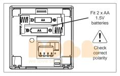
Fit the two supplied AA batteries. The battery compartment is marked with a plus and minus sign. Ensure that each battery is correctly aligned. The SES 302/303 will now power up.
