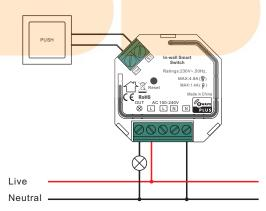
**NOTE:** Switch connected to the S1 terminal activates the basic functionality of the switch (turning the light on/off) and starts the inclusion/exclusion mode (Add/Remove).
