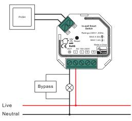
**NOTE:** Switch connected to the S1 terminal activates the basic functionality of the switch (turning the light on/off) and starts the inclusion/exclusion mode (Add/Remove).
