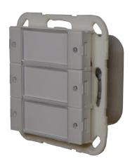
ZHC5002 is a Z-Wave coupler module for GIRA pushbuttons. The module is designed for interfacing a GIRA push button sensor module (GIRA push button sensor 2, type 2003) with two 10-pole connectors to a Z-Wave network.
