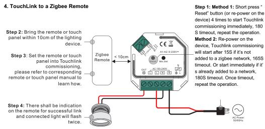
Note: 1) Directly TouchLink (both not added to a ZigBee network), each device can link with 1 remote.
