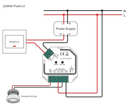
This phase dimmer adopts leading edge dimming (forward phase control) or trailing edge dimming (reverse phase control), two versions are available for choosing. Please make sure the connected loads support the control type you choose. Please refer to the user manual of the load or consult the supplier of the load.
