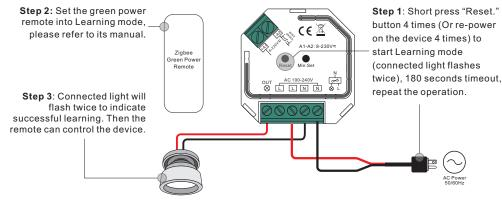
Note: Each device can learn to max. 20 zigbee green power remote.
