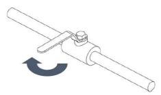
Valve should open/close easily by hand, without the use of any tools. The valve handle should be perpendicular to the pipe, which means the valve is closed.
