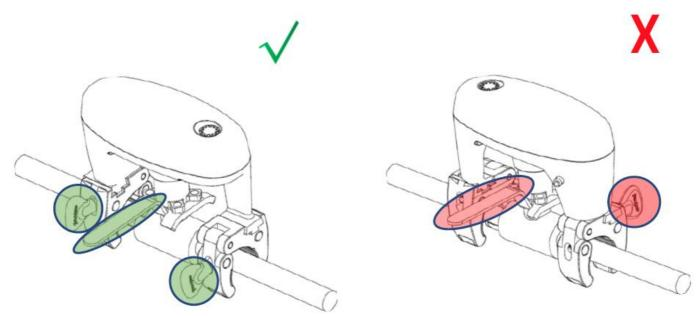
Installation Step 5: Check if the folk is coupled and aligned with th valve handle correctly
