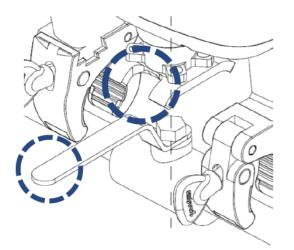
Installation Step 4: Check if the clamps and the valve handle are facing the same side
