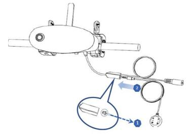
Installation Step 8: Connect the power supply to the BVS, lock the ring connector tightly and plug into the outlet
