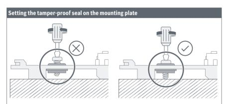
The siren is protected by a tamper-proof seal. This will trigger an alarm if the siren is removed from the wall of the house without authorisation. After attaching the mounting plate to the wall of the house, the tamper-proof seal must be set correctly. To do this, turn the adjusting screw on the contact clockwise with a screwdriver until the tip touches the wall of the house.
