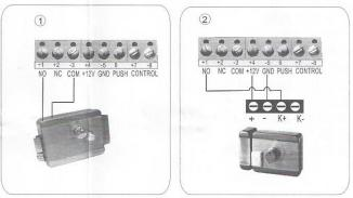
Attention! then electronically controlled lock must be transferred to 0 seconds delay, to prevent burning of electric locks.
