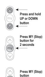
**NOTE:** Blind should be stationary prior to activating intermediate position function. If slats are actively moving (in-motion), the **MY (Stop)** button should be pressed twice.
