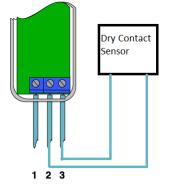
You can wire any dry contact sensor output to Terminal #2 and #3 (it doesn't matter which terminal is wired to where). Dry contact terminals are only looking for Open/Close control which will have Door / Window Sensor 7 report its status depending on the state of the dry contact output to Door / Window Sensor 7.
