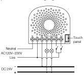
Note: The "IN" terminal should be connected to the "-" of DC 24V input.
