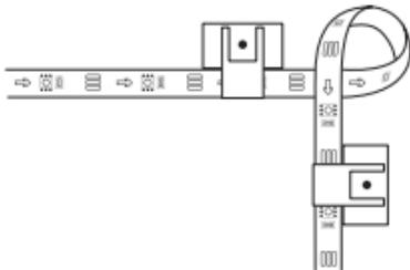
d. Connect the power brick to the strip and the adapter. Peel off the protective film on the tape to stick it on.
