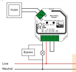
**NOTE:** Switch connected to the S1 terminal activates the basic functionality of the dimmer (turning the light on/off, dimming) and starts the inclusion/exclusion mode (Add/Remove).
