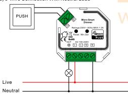
NOTE: Switch connected to the S1 terminal activates the basic functionality of the dimmer (turning the light on/off, dimming) and starts the inclusion/exclusion mode (Add/Remove).
