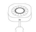
2. Use the included screws to mount the back plate of the device on the wall
