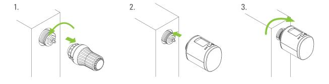
Installation at the radiator with Adapter
