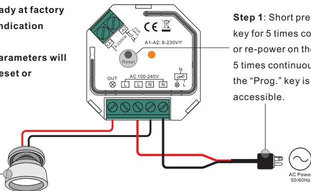
**Step 1:** Short press "Reset." key for 5 times continuously or re-power on the device for 5 times continuously if the "Prog." key is not accessible.
