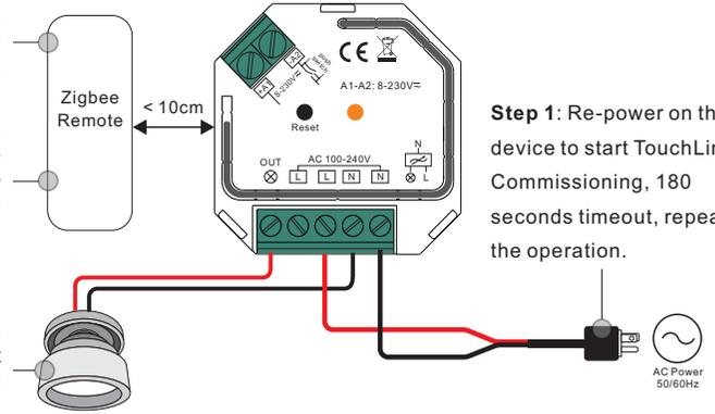
**Step 1:** Re-power on the device to start TouchLink Commissioning, 180 seconds timeout, repeat the operation.
