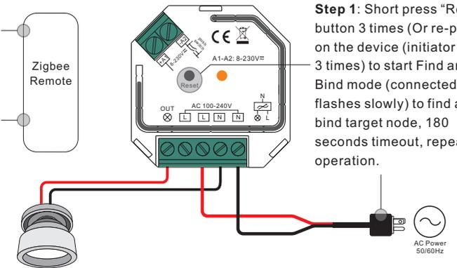
**Step 1:** Short press "Reset." button 3 times (Or re-power on the device (initiator node) 3 times) to start Find and Bind mode (connected light flashes slowly) to find and bind target node, 180 seconds timeout, repeat the operation.
