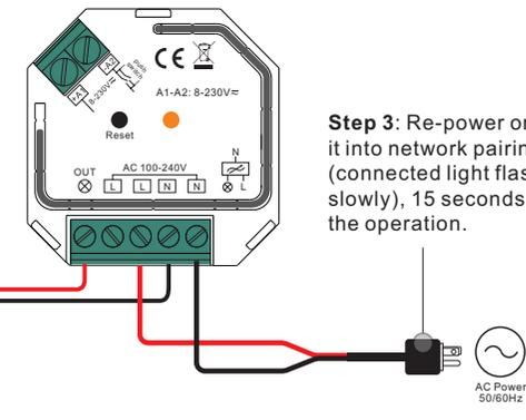
**Step 3:** Re-power on the device to set it into network pairing mode (connected light flashes twice slowly), 15 seconds timeout, repeat the operation.
