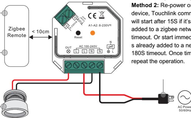
**Step 1: Method 1:** Short press "Reset" button (or re-power on the device) 4 times to start Touchlink commissioning immediately, 180 S timeout, repeat the operation.
