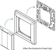
the frame and control part to the bracket in sequence
