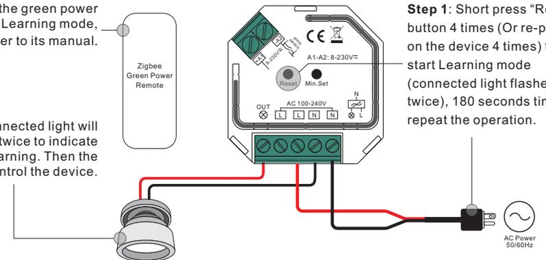
**Step 1:** Short press "Reset." button 4 times (Or re-power on the device 4 times) to start Learning mode (connected light flashes twice), 180 seconds timeout, repeat the operation.
