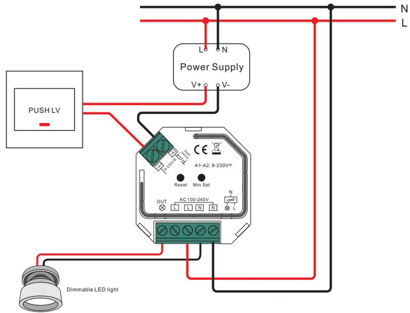
This phase dimmer adopts leading edge dimming (forward phase control) or trailing edge dimming (reverse phase control), two versions are available for choosing. Please make sure the connected loads support the control type you choose. Please refer to the user manual of the load or consult the supplier of the load.
