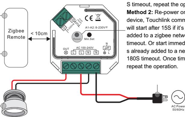
**Step 1: Method 1:** Short press "Reset" button (or re-power on the device) 4 times to start Touchlink commissioning immediately, 180 S timeout, repeat the operation.
