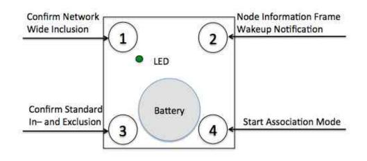
Button 1 - Network Wide Inclusion: The device can be included into a Z-Wave network from any physical location in the network. This requires a primary controller supporting Explorer Frames. This mode lasts for 20 seconds and stops automatically. Any button press stops the mode as well.
