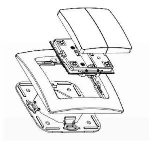
The device can be mounted on every dry and flat surface using either screws or double side adhesive. First the mounting base is fixed on the wall. Next step the switch frame is placed on the 2 frame and the electronic insert is used to fix the frame to the mounting base as shown on the image. Finally the switching paddle(s) are mounted on the electronic base.
