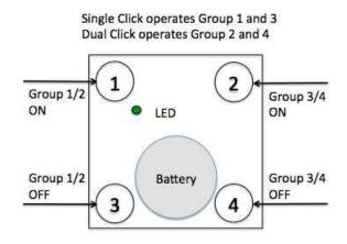
**Control with single buttons** In this mode a group of devices is controlled by a single button: single click turns 'ON'; double click turns 'OFF' devices in the group. In case dimmers are controlled, holding down the button will dim up, click and hold down will dim down the load. The group number corresponds to the button label.
