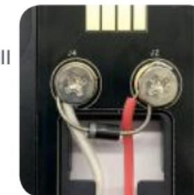
**i** If you have a **digital doorbell**, connecting the diode the wrong way won't do any harm. If your existing doorbell doesn't ring, just reverse the diode.
