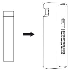
Use the adhesive strip to mount the devie on the wall or the window frame.
