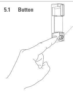
**Note:** To use the low push button in the housing of the Door/ Window Contact, use a paper clip or a similar thin item.
