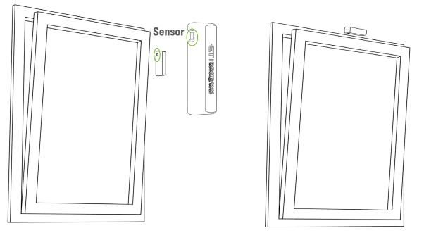
Select a suitable place for the Door/Window Contact on the side of the windor or the door. The ideal distance to the sensor is 3 mm. The sensor must be aligned with the window or the door.
