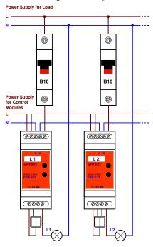
The descriptions of the screw terminals are printed on the adapter label. The letters "IN" indicate input for powering the load device. The "Q1" letters indicate the relay output.
