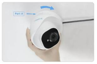
Step 4. Once the camera is installed, you can adjust the angle up & down 70 degrees or 360 degrees horizontally.
